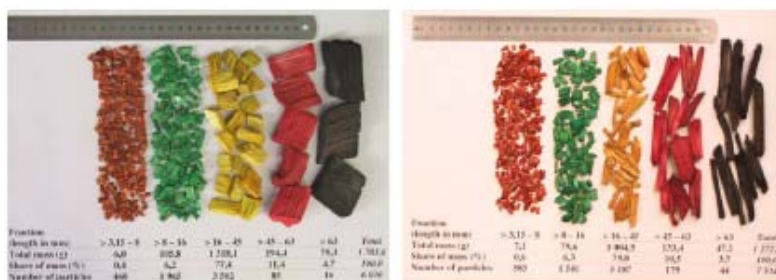
Fig. 2. Example of particles in the manually prepared and coloured standard wood chip sample (SF1, left) and hog fuel sample (SF2, right).
