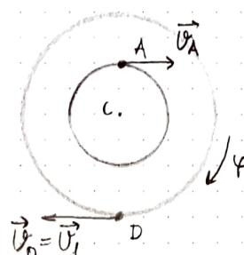
$$V_1 = R\dot{\varphi} \Rightarrow \dot{\varphi} = \frac{V_1}{R} \quad (6)$$
