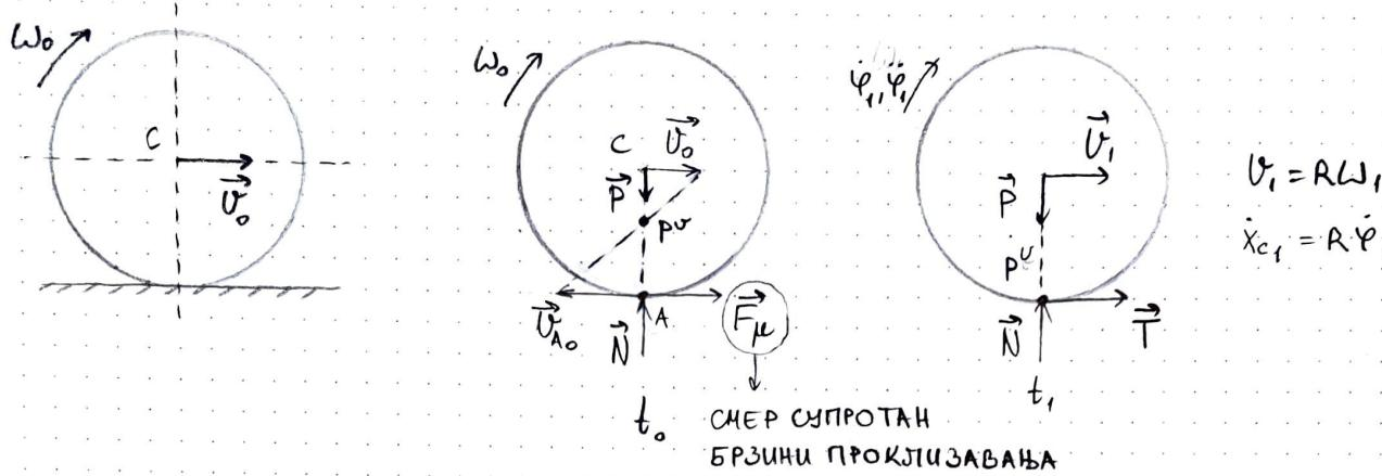
$$\checkmark \frac{d\dot{x}_c}{dt} = M_{C_2}^S = -RF_{\mu}, \quad F_{\mu} = \mu N$$
