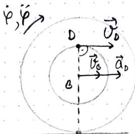
$$\begin{aligned} \dot{\theta}, \ddot{\theta} \\ \vec{v}_C &= \vec{v}_D = \vec{v}_C \\ &= R \dot{\theta} \end{aligned}$$
