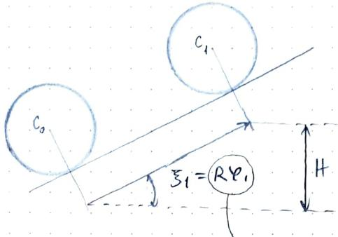
$$A_{0-1}(\vec{N}) = k \int_0^{\varphi_1} N d\varphi \\ = kN \int_0^{\varphi_1} d\varphi$$
