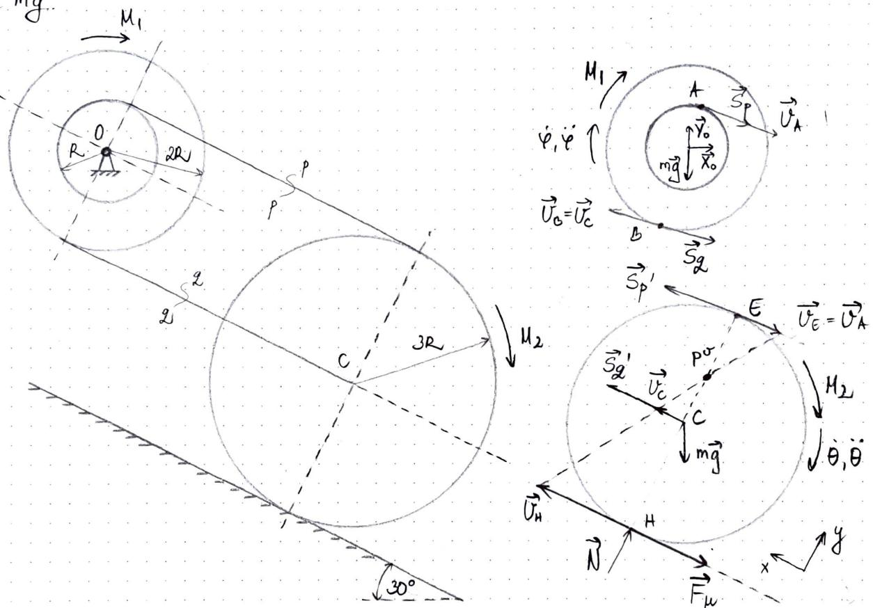
$$\left. \begin{aligned} \ddot{\phi}_2 &= M_{2z} = R S_p - 2R S_q + M_1 \\ \dot{\phi}_2 &= J_{2z} \dot{\phi} = m i_0^2 \dot{\phi} = 2mR^2 \dot{\phi} \Rightarrow \frac{d\phi_2}{dt} = 2mR^2 \ddot{\phi} \end{aligned} \right\} \quad \begin{aligned} 2mR^2 \ddot{\phi} &= R S_p - 2R S_q + M_1 / R \\ 2mR \ddot{\phi} &= S_p - 2S_q + \frac{M_1}{R} \quad (1) \end{aligned}$$
