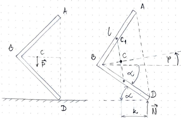
$$\overline{BC}\sqrt{2} = \frac{l}{2} \Rightarrow \overline{BC} = \sqrt{\frac{l^2}{4}}, \overline{CC_1} = \overline{BC}$$
