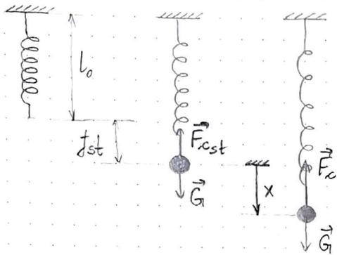
$$c = \frac{0,5\text{N}}{1\text{cm}} = 50 \frac{\text{N}}{\text{m}}$$
