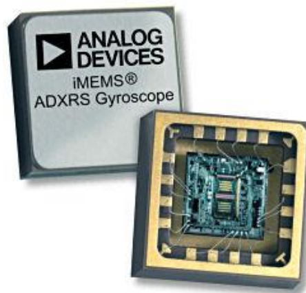
Figure 4-8 MEMS gyro
