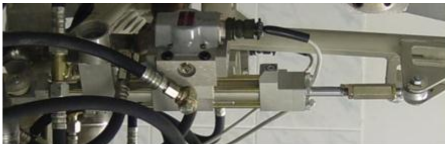
Figure 2-14 Actuator: control valve + cylinder
