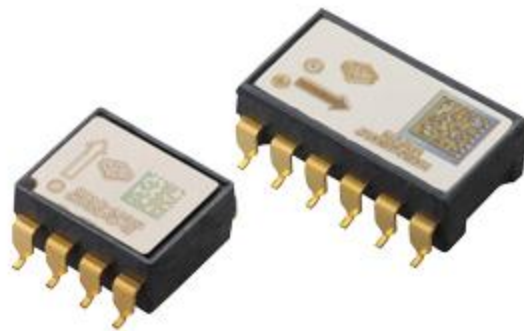
Figure 4-3 MEMS accelerometer
