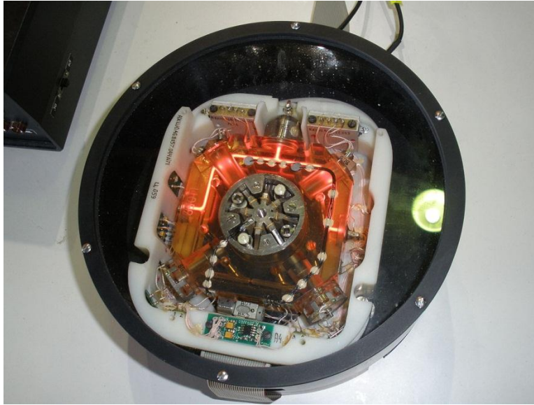
Figure 4-7 Ring laser gyro
