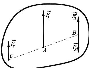
$$\begin{aligned}\vec{F}_l &= \vec{F}_r + \vec{F}'_2 \\ (\vec{F}_l, \vec{F}_2) &\sim (\vec{F}_r, \vec{F}'_2, \vec{F}_2) \\ (\vec{F}_l, \vec{F}_2) &\sim \vec{F}_r \\ \vec{F}_l &= \vec{F}_r - \vec{F}_2 \\ \vec{F}_r &= \vec{F}_l + \vec{F}_2\end{aligned}$$
