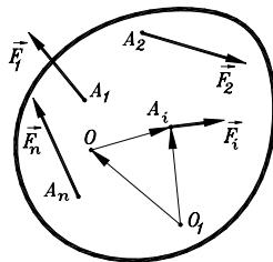
$$\begin{aligned}\vec{M}_o &= \sum_{i=1}^n \vec{M}_{o_i}(\vec{F}_i) = \sum_{i=1}^n \overrightarrow{OA_i} \times \vec{F}_i \\ \vec{M}_{o_i} &= \sum_{i=1}^n \vec{M}_{o_i}(\vec{F}_i) = \sum_{i=1}^n \overrightarrow{O_1A_i} \times \vec{F}_i \\ \overrightarrow{O_1A_i} &= \overrightarrow{O_1O} + \overrightarrow{OA_i} \\ \vec{M}_{o_i} &= \sum_{i=1}^n \overrightarrow{O_1O} \times \vec{F}_i + \sum_{i=1}^n \overrightarrow{OA_i} \times \vec{F}_i\end{aligned}$$
