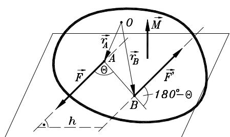
$$\begin{aligned}\vec{M}_o &= \vec{M}_o(\vec{F}) + \vec{M}_o(\vec{F}') \\ \vec{M}_o &= \vec{r}_A \times \vec{F} + \vec{r}_B \times \vec{F}' \\ \vec{r}_A &= \vec{r}_B + \overrightarrow{BA}, \quad \vec{F}' = -\vec{F} \\ \vec{M}_o &= (\vec{r}_B + \overrightarrow{BA}) \times \vec{F} - \vec{r}_B \times \vec{F}. \\ \vec{M}_o &= \overrightarrow{BA} \times \vec{F}\end{aligned}$$
