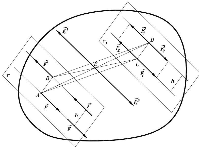
$$\begin{aligned}\vec{F}_r^I &= -\vec{F}_r^2, & F_r^I &= F_r^2 \\ (\vec{F}', \vec{F}_2) &\sim \vec{F}_r^I & \text{and} & (\vec{F}, \vec{F}_2') \sim \vec{F}_r^2 \\ (\vec{F}, \vec{F}') &\sim (\vec{F}_l, \vec{F}_l', \vec{F}_r^I, \vec{F}_r^2)\end{aligned}$$
