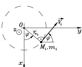
$$L_x = \vec{L}_O \cdot \vec{i} = \sum_{i=1}^n m_i (y_i \dot{z}_i - z_i \dot{y}_i), \dots,$$
