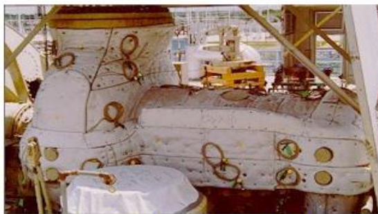
A turbine warming system installed on a steam turbine
