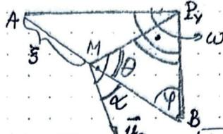
$$\overline{MP_v}^2 = \overline{BM}^2 + \overline{BP_v}^2 - 2\overline{MB} \cdot \overline{BP_v} \cos \varphi$$
