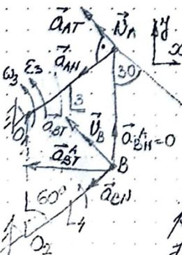
$\vec{v}_A = \vec{v}_B$  ;  $\vec{v}_A = \vec{v}_C$  , odnosno  $\boxed{\vec{v}_{cp} = \vec{v}_A}$  ( $\angle(Cy, \vec{v}_{cp}) = 30^\circ$ )
