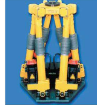
Fanuc F-200iB parallel kinematics
