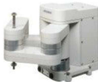
Mitsubishi RP (repeatability 5 micron, payload 5 kg)
