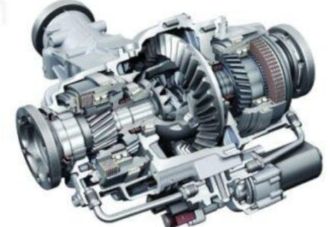
Torque Vectoring Differential
