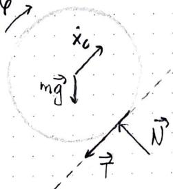
$$(7) \rightarrow (5), (6) \Rightarrow 2R\omega_0 - \frac{2\sqrt{2}}{3}gt_1 = R\left(\omega_0 + \frac{\sqrt{2}}{6} \frac{g}{R} t_1\right)$$
