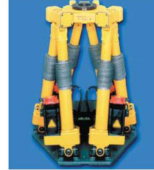
Fanuc F-200iB parallel kinematics
