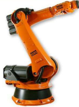
Kuka 150_2 (series 2000) open kinematic chain (rigid bodies connected by joints)
