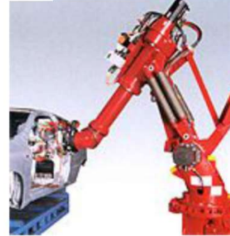
Comau Smart H4 closed kinematic chain
