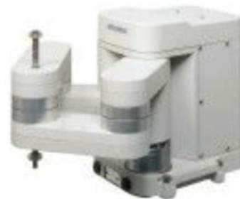
Mitsubishi RP (repeatability 5 micron, payload 5 kg)
