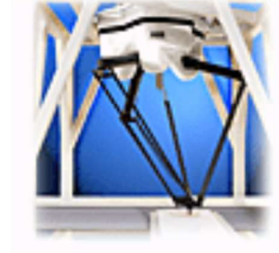
ABB Flexpicker (150 pick-and-place operations/minute)
