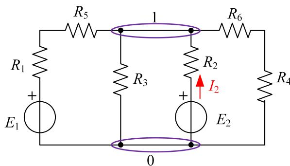
$$I_2 = \frac{V_0 - V_1 + E_2}{R_2} = \frac{9 - 5,7273}{100} = 0,033 \text{ A} = 33 \text{ mA}$$
