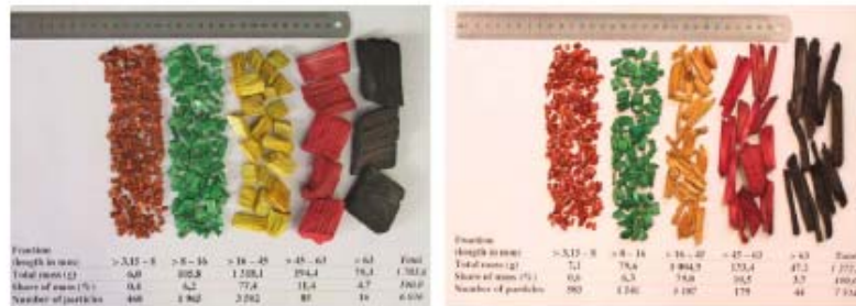
Fig. 2. Example of particles in the manually prepared and coloured standard wood chip sample (SF1, left) and hog fuel sample (SF2, right).
